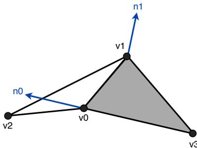
Figure 1: The important geometric values for each edge in McGuire and Hughes' method:  $v_0$ ,  $v_1$ ,  $v_2$ , and  $v_3$  are vertices on two polygons that share an edge.  $n_0$  and  $n_1$  are the vertex normals for  $v_0$  and  $v_1$ , respectively.  $v_3$  may not exist in the case of a boundary edge.
