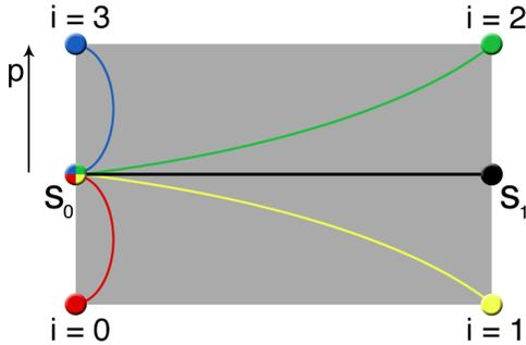
Figure 2: Depending on the  $i$  value, the output point is calculated using the two screen-space edge points and the perpendicular vector.
