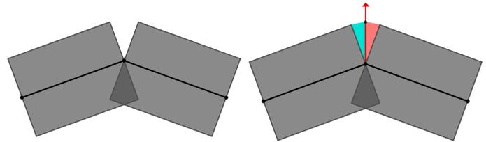
Figure 4: On the left, two thick screen-space edge quads connect to create a visible gap. Using the screen-space projection of the vertex normal they share, the gap can be filled with a cap formed from one half-cap from each edge (one blue, one red), as seen on the right.
